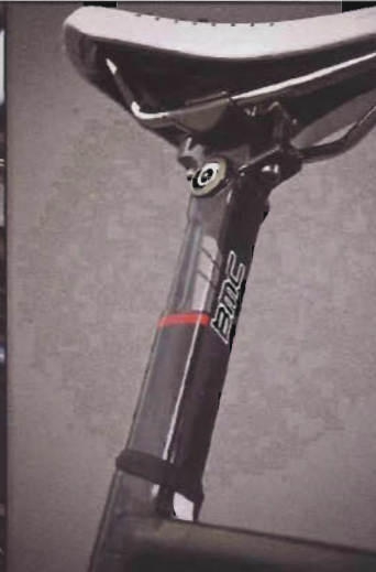
Don't underestimate the clever configuration of the seatpost on this bike. It won't be long before other manufacturers try to mimic this cammed fastening.
