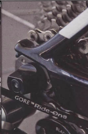
The drop-outs are a continuation of the rectangular profile of the chainstays. BMC has really isolated the driving forces through the rear end by doing this...
