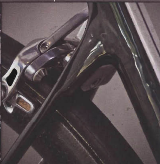
BMC has included an aluminium reinforcement for the clamp area of the rear brake. The seatstays are thin and contribute to the ride quality and this insert (which goes through to the other side) means the calliper won't affect the frame's strength.
