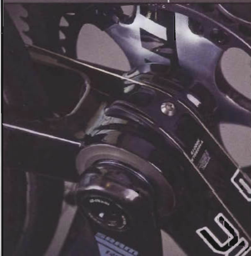
Cables are sent to their respective regions with the most direct path possible – unlike the Pinarello for example, where there was a degree of compromise. With BB30 cranksets the spacers must be absolutely correct to achieve the right bearing compression.
