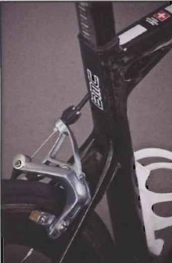
Another angle of the low seatstay junction and the clamp-free area of the seat tube. By not having a round profile, the frame provides a degree of flex which is intentional.
