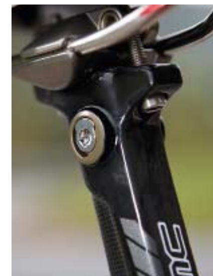
▶ Marcel is a fan of the BMC seatpost's innovative clamp-free cam-lock design
